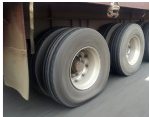
▲ Underinflation – friction causes heat.
