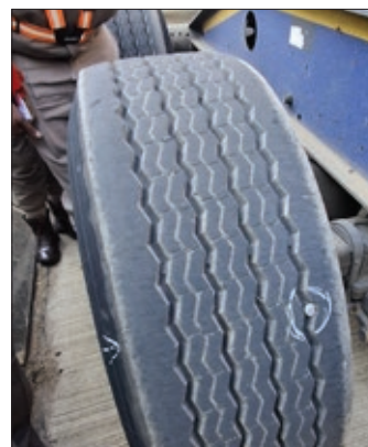
▲ A metal object in the tread may damage the road surface or be a danger. Remove the object. - Reg 212 (E)
