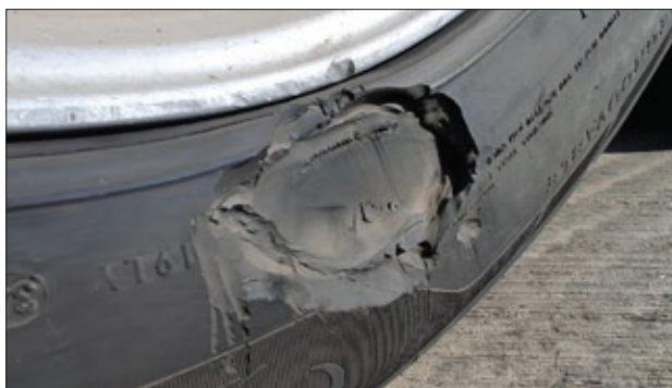
▲ This tyre has a massive cut/break on the outside of the tyre measuring more than 25 mm and the cords are exposed. Take it off - Reg 212 (L)
