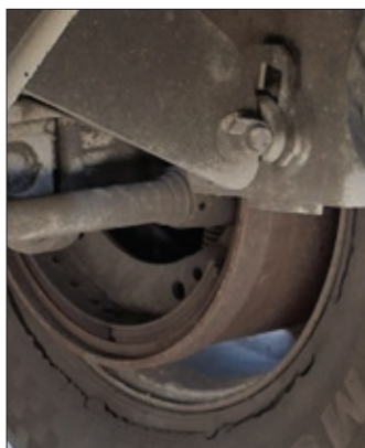
▲ Another tyre with a huge cut on the outside of the tyre measuring more than 25 mm. This is obvious for goodness sake. Get it off. - Reg 212 (L)
