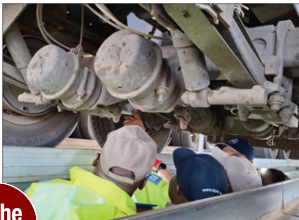
▲ Condition of tyres can be inspected closely in the pit. Often the inner tyre on a set of twins has faults that the cops won't spot on the road.
