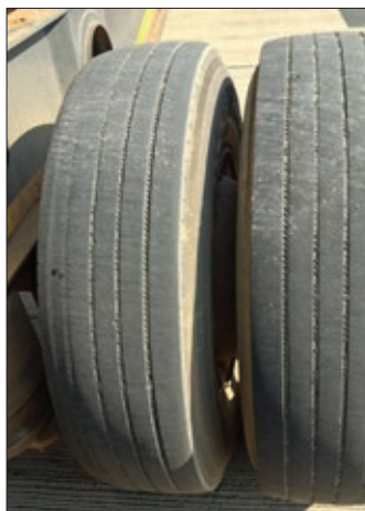
▲ Tread depth has reached the Tread Wear indicator (TWI). These tyres are smooth and illegal - (Reg 212 J)
