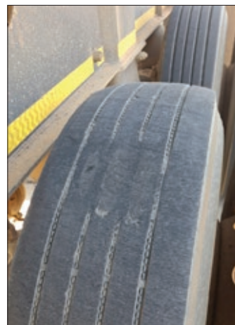
▲ Again, the tread depth has gone beyond the Tread Wear Indicator making this tyre illegal. - (Reg 212 J)
