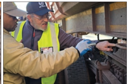
▲ Getting up close... Manie Roux from Jost explains the workings of the Fifth Wheel. You'd be surprised at how many faults are picked up on Fifth Wheels, an all-too often overlooked safety component which, when it fails, leads to catastrophic consequences. Safety latches are often missing and replaced with blou-draad - a definite recipe for disaster.
