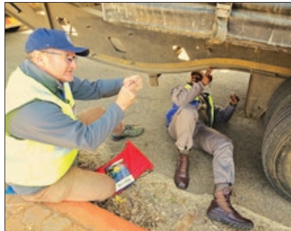
▲ Craige Proctor-Parker of Accident Specialist , guides a delegate in tracing the ABS cables under a trailer.
