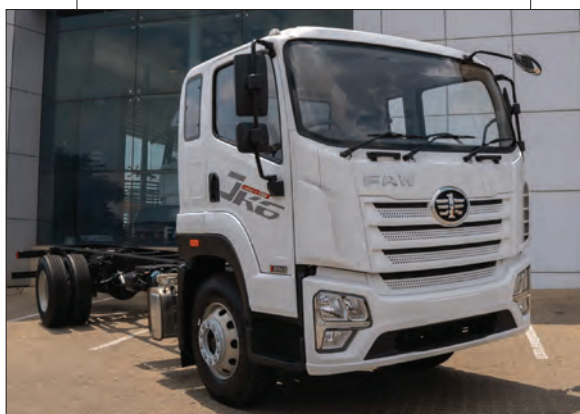
▲ The FAW JK6 16.260 chassis-cab ready for a body of choice. There are two variants, one with a manual gearbox and the other with an Automated Manual Transmission.
