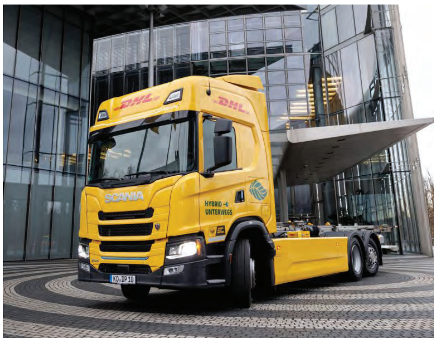
▲ Electric engine with a backup diesel/petrol/biofuel genny - the DHL Scania hybrid truck is currently proving its long-haul mettle in Germany.
