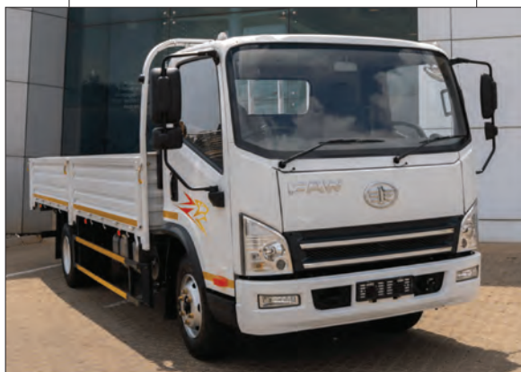
▲ The light-commercial FAW 4.1 10 FL-MT with a dropside body can haul 2.5-tonnes with economy and comfort.
