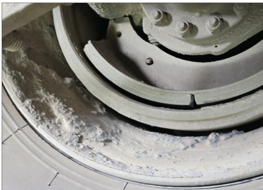
▲ Brakes shoe is not touching the drum – the gap is too big meaning the settings are wrong. NO BRAKES!
