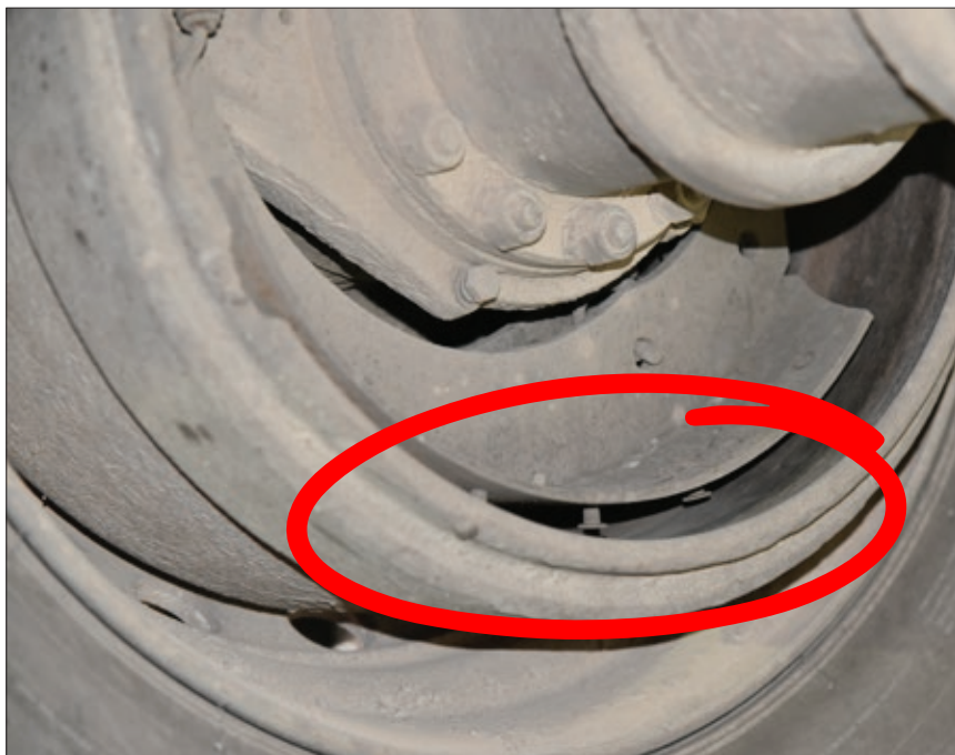
▲ No lining on the brake shoes – again NO BRAKES! (Top and bottom)
