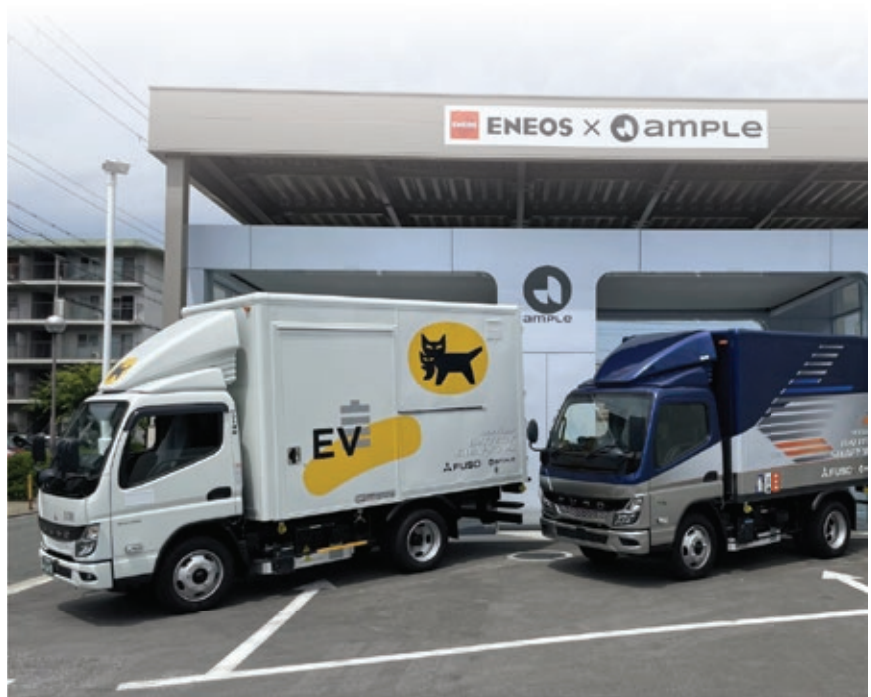
▲ Running on swappable batteries fitted by robots at an Ample EV battery swapping station – two new eCanter derivatives (the one on the left operated by Yamato Transport Co).
