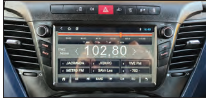
▲ The 7" colour display screen. The rear camera also feeds to this screen.
