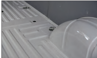
▲ Floor mounted tie down points to secure loads
