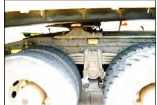
▲ A fifth wheel behind the drive axle centre line means mass transfer from the front axle to behind the drive axle – and very poor mass distribution
