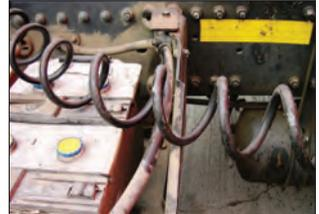
▲ Dirty brake pipes fouling the battery cradle are a sure indicator of lack of attention to the rest of the braking system
