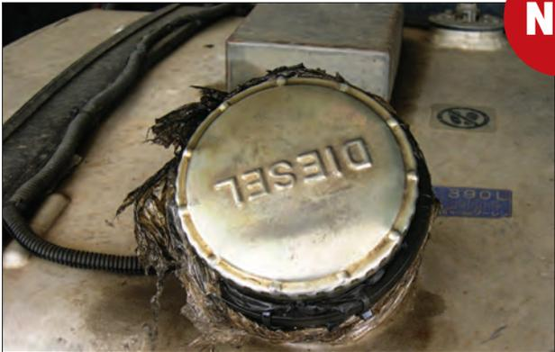
▲ Fuel is the biggest cost in transport but a tank leak countermeasure is with a 'vrot' plastic bag
