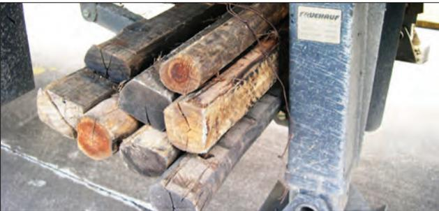
▲ These logs used for trailer supports are tied down with loose rusty wire and can fall off to create a crisis for other road users
