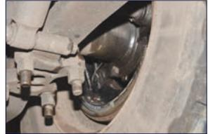
▲ Oil and muck all over the brake drums. Might as well be braking on ice.
