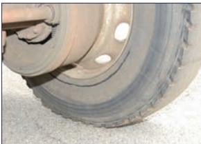
▲ Shocking. Totally bald tyre with a huge cut on the inner wall. A blowout just waiting to kill.
