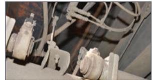
▲ When slack adjusters are incorrectly set such as is seen here, this is a sure sign of imbalanced – and invariably no braking.
