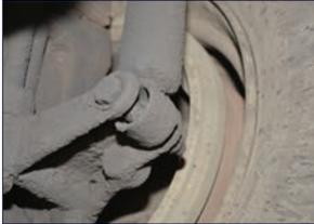
▲ The bush is missing from this shock absorber rendering it totally useless in its function.
