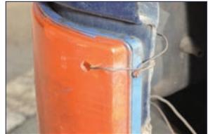
▲ The use of 'bloudraad' on small things is a sure sign of bigger faults on a rig.
