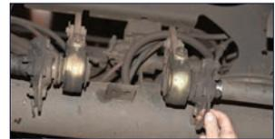
▲ The adjustment bracket is supposed to be for an automatic slack adjuster (Ling Zong) but the operator has replaced both automatic slack adjusters with manual slack adjusters making this trailer illegal. Also note the camshaft is moving excessively
