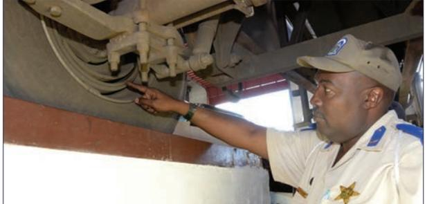
▲ One of the traffic officials shows the huge gap between the brake lining and the drum – impossible to brake. Total fail. This is common on many trucks we take off for testing.
