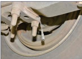
▲ An ABS sensor is disconnected rendering the ABS system useless.
