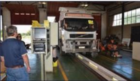
▲ One of the rigs being taken over the brake roller tester in the test centre.
